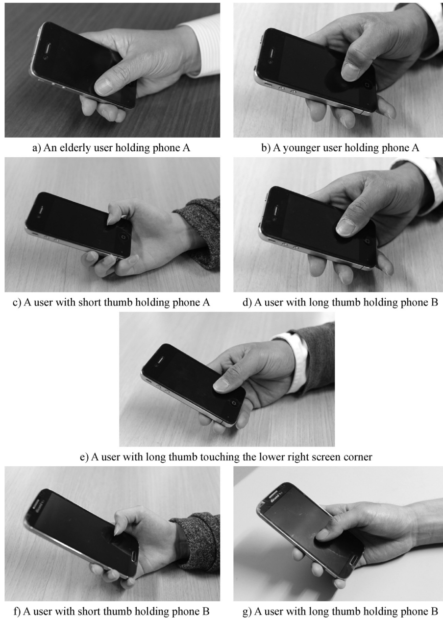
Fig. 7. Phone-holding postures for the smaller phone (phone A) and larger phone (phone B).
